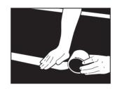
3. Tape all joins with single sided waterproof tape and press firmly into place.
